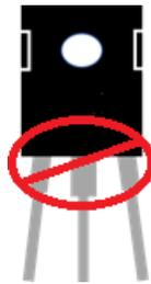
Figure 3 Sideways bending may cause damage
