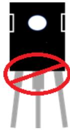
Figure 3 Sideways bending may cause damage
